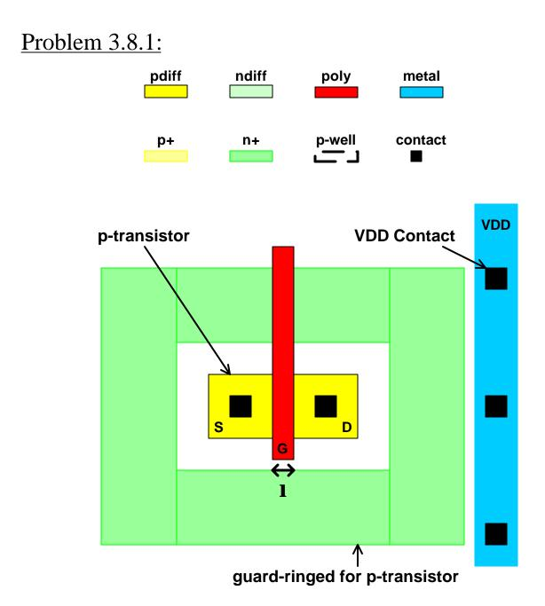
Note: in p-well process, the substrate is n-type.
