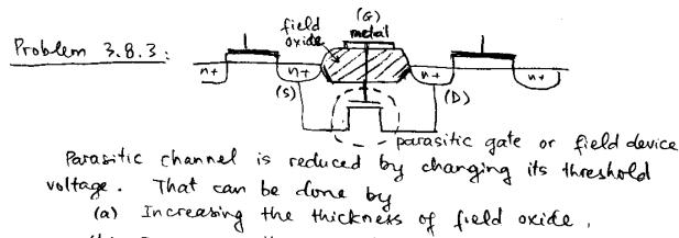
(b) Increasing the impurity concentration under the field oxide
