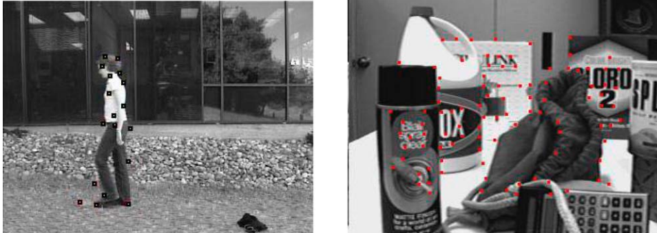
Figure 4. Sample outputs of feature selection algorithm run on a selected portion of the images. Features are denoted by black squares with white centers in the left image, and by filled dark squares in the right image.
