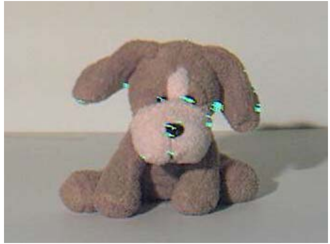
Figure 8. 148 features are selected by automatic threshold adjustment (FS-AUTO) under default lighting conditions.
