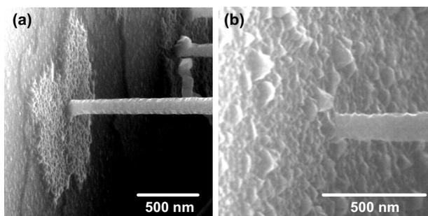
**Figure 3.** (a) Detail of a disc formed along the (111) sidewall surrounding the impinging end of an Au-nucleated nanowire. (b) Detail of the impinging end of a Ti-nucleated Si nanowire making a rigid connection with the opposing sidewall.
