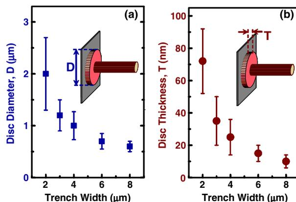
**Figure 4.** (a) Diameter and (b) thickness of discs extending from impinging nanowires along the sidewalls of trenches after bridging as a function of trench width.
