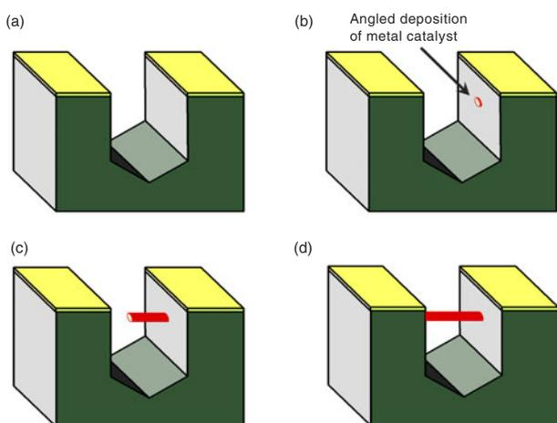
**Figure 1.** Schematic diagrams of (a) trench formation, (b) catalyst deposition, (c) lateral nanowire growth, and (d) bridging across trench.
