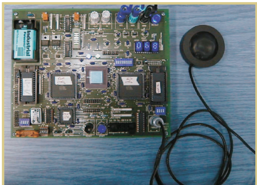
Figure 1. Wearable biomedical acoustic sensor demonstration system.
