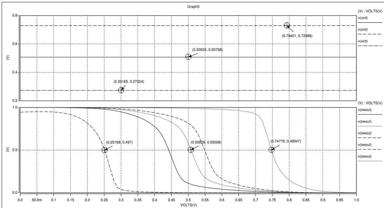
Figure 2: Inverter sizing based on inverter output feedback and on DC input voltage sweep.
