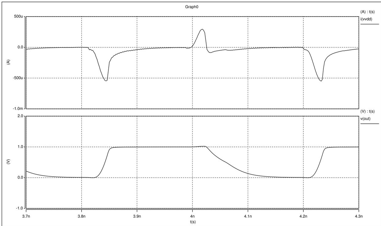
Figure 11: Single charge-discharge cycle and corresponding power supply current for a single inverter in the ring oscillator (switching threshold  $3V_{DD}/4$ ).
