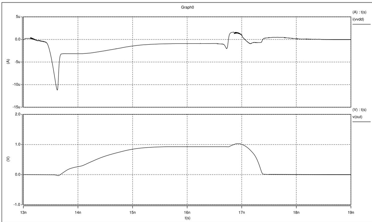
Figure 10: Single charge-discharge cycle and corresponding power supply current for a single inverter in the ring oscillator (switching threshold  $V_{DD}/4$ ).
