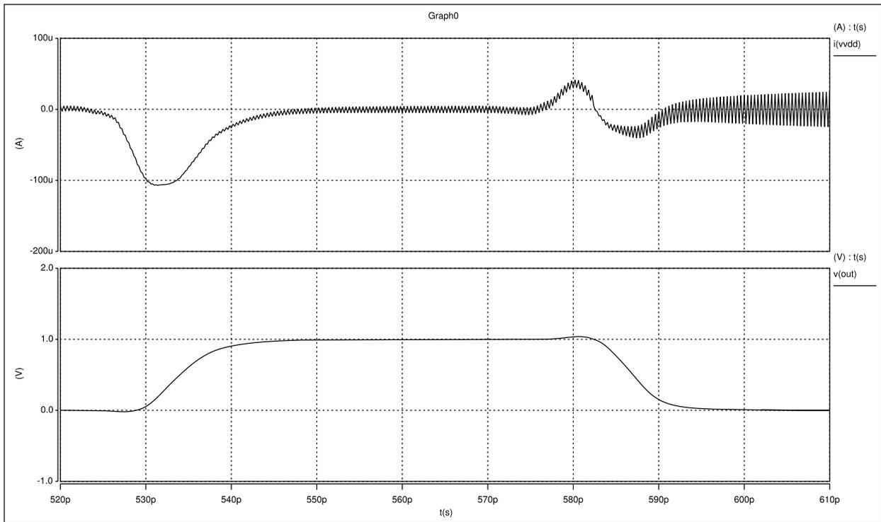
Figure 9: Single charge-discharge cycle and corresponding power supply current for a single inverter in the ring oscillator (switching threshold  $V_{DD}/2$ ).
