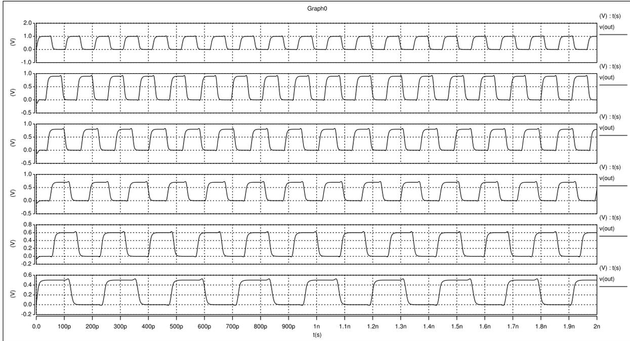
Figure 3: Ring oscillator waveforms at different supply voltages ( $\frac{V_{DD}}{2}$  switching threshold).
