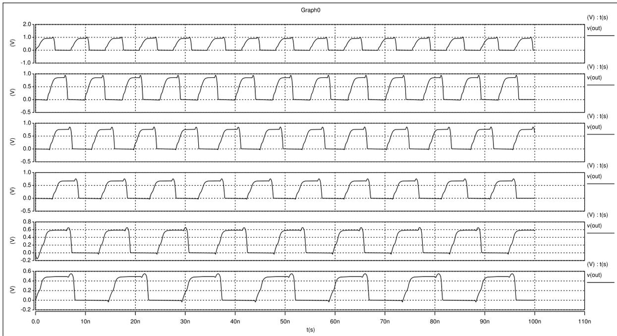
Figure 4: Ring oscillator waveforms at different supply voltages ( $\frac{V_{DD}}{4}$  switching threshold).
