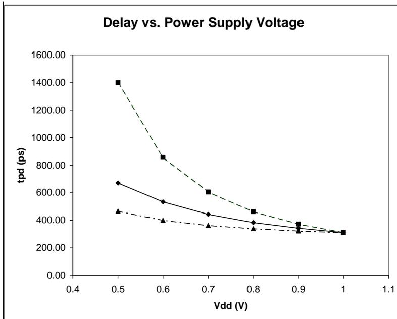
Figure 7: Inverter delay versus supply voltage ( $\frac{V_{DD}}{4}$  switching threshold).
