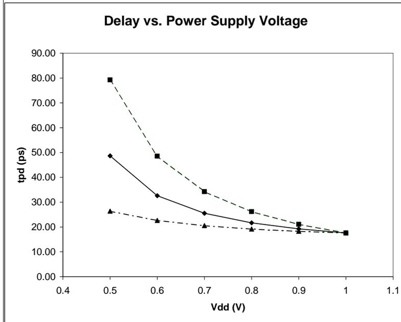
Figure 8: Inverter delay versus supply voltage ( $\frac{3V_{DD}}{4}$  switching threshold).
