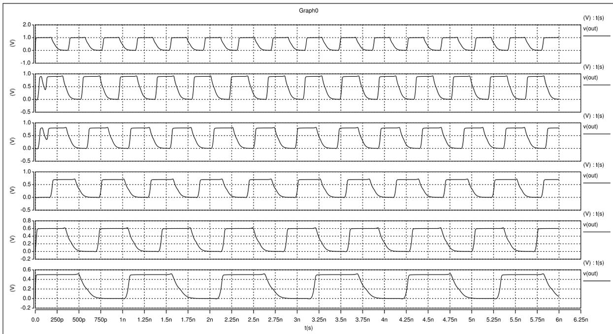
Figure 5: Ring oscillator waveforms at different supply voltages ( $\frac{3V_{DD}}{4}$  switching threshold).
