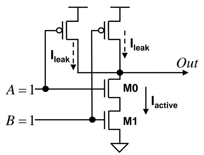
•  $I_{active}/I_{leak}$  ( $I_{on}/I_{off}$ ) ratio can be small in subthreshold
