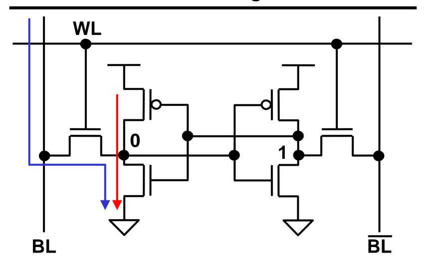
Leakage paths can degrade read and write noise margins
