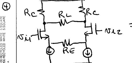
$$\begin{aligned} & DM \parallel \text{2 CKT} \\ & R_{C2} \parallel R_{L2} \parallel R_{D2} \parallel \frac{R_E}{2} \quad Adm = -G_m R_o \\ G_m &= \frac{q_m}{1 + q_m \frac{R_E}{2}} \\ R_o &= R_C \parallel R_{L2}/2 \parallel R_{D2} \parallel \frac{\infty}{\infty} \\ Adm &= -\frac{q_m (R_C \parallel R_{L2}/2)}{1 + q_m R_E/2} \end{aligned}$$
