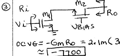
$$\begin{aligned} & |R_i \rightarrow \infty| \\ G_m &= qm_1 = \sqrt{2(90)(100)(250)} \approx 2.1 \text{ mA/V} \\ R_o &\approx (q_{m2} + q_{mb2}) R_{o2} R_{o1} = q_{m2}(1+\lambda) R_{o2} R_{o1} \\ R_{o1} &= R_{o2} = \frac{1}{\lambda I} = \frac{10}{250} = 40 \text{ k}\Omega \\ R_o &\approx 2.1 (1+0.1)(40\text{k})^2 \approx 3.7 \text{ meq} \Omega \end{aligned}$$
