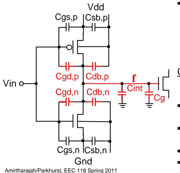
Assume input transition is fixed, then delay determined by output
