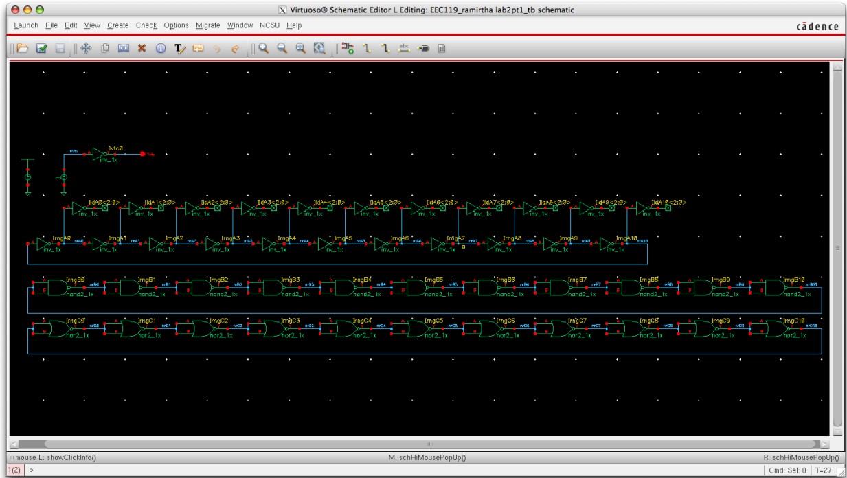
Figure 4: Three ring oscillator testbench schematic.
