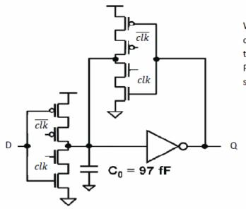
We want the latch to be transparent when clk is positive, so we put clk at the gates of the NMOS's and clk\_bar at the gates of the PMOS's. The feedback inverter makes it static instead of dynamic.
