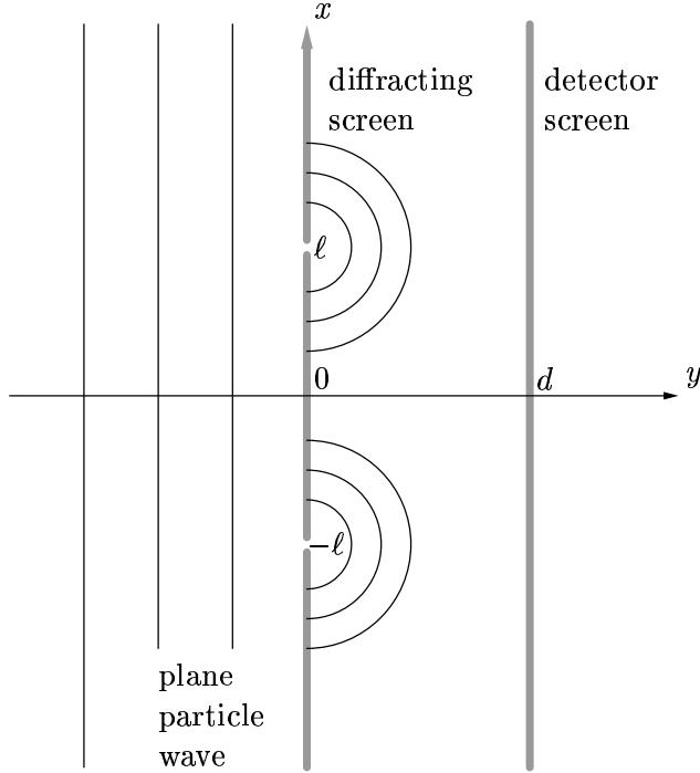
Figure 1: Two-slit particle diffraction experiment.
