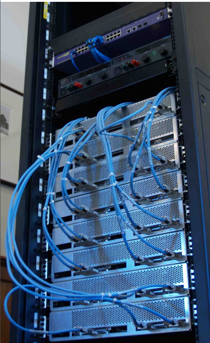
RAMP Blue, January 2007 ▪ 256 RISC cores @100MHz ▪ Works! Runs UPC version of NAS benchmarks.
