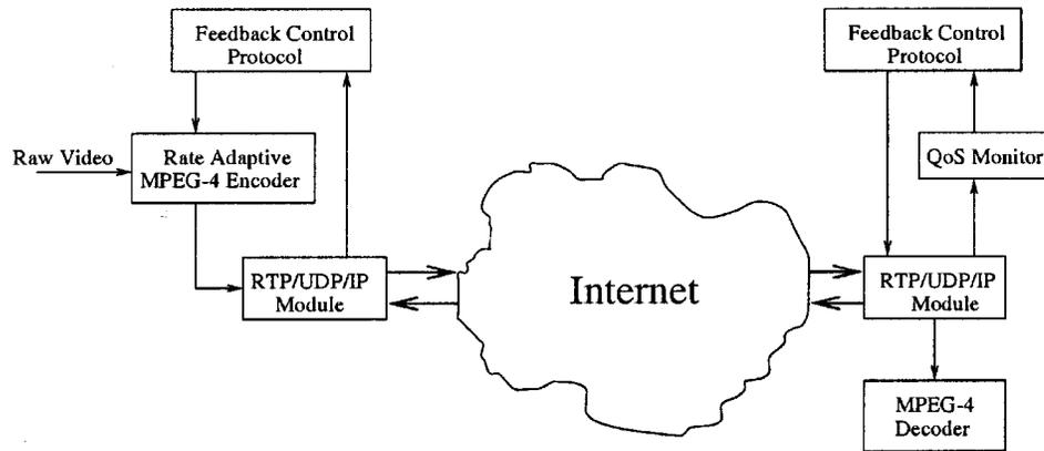
Fig. 1. An end-to-end architecture for transporting MPEG-4 video.
