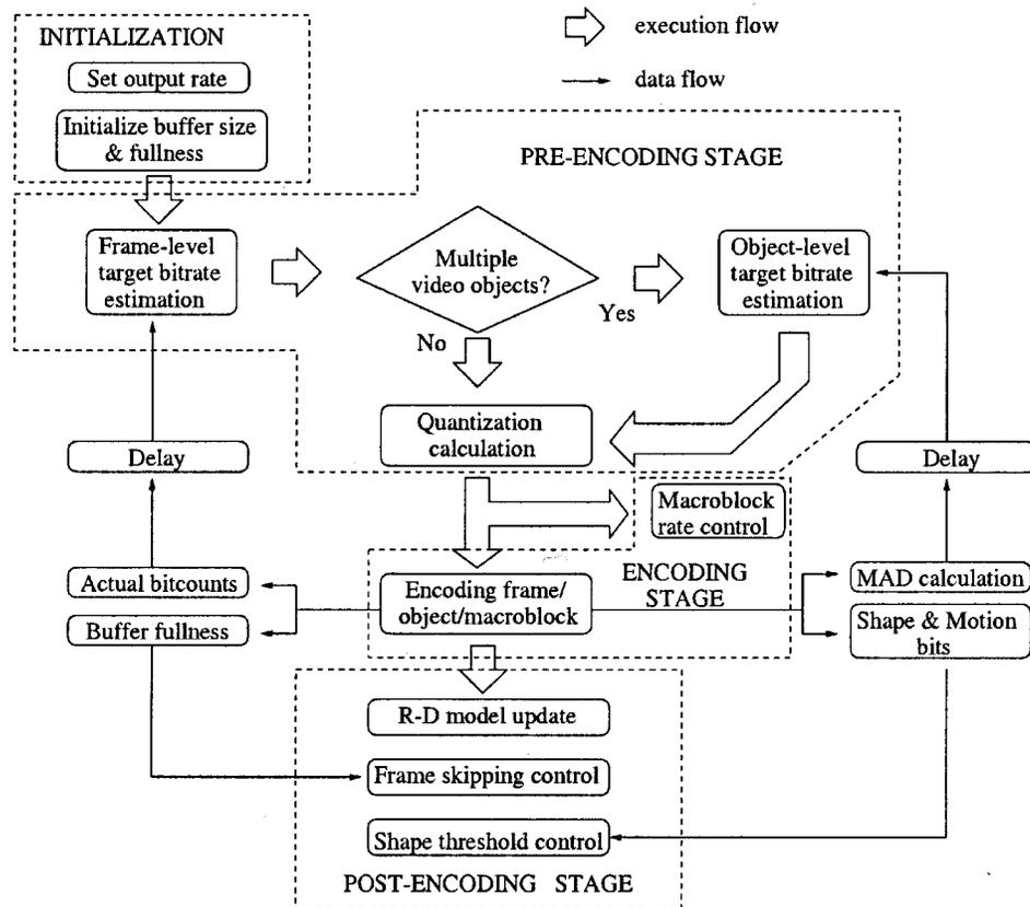
Fig. 6. Block diagram of our encoding rate-control scheme.
