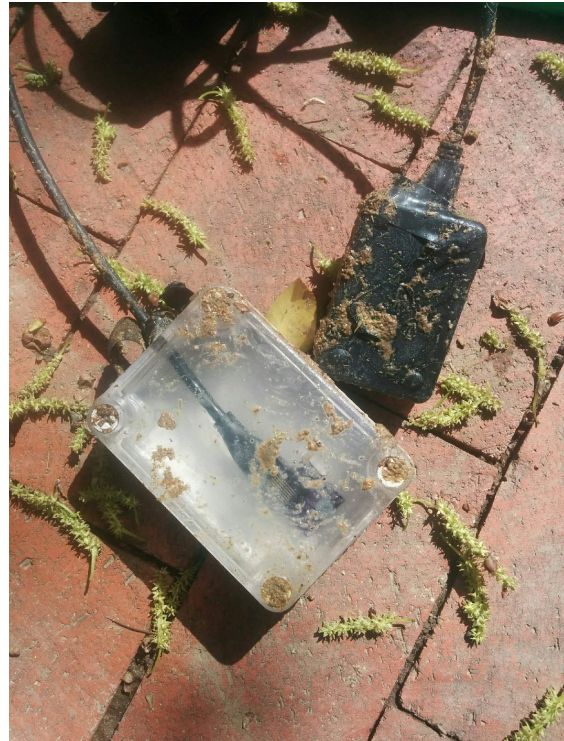
Figure 9: IR and RFID cases after removal from field test
