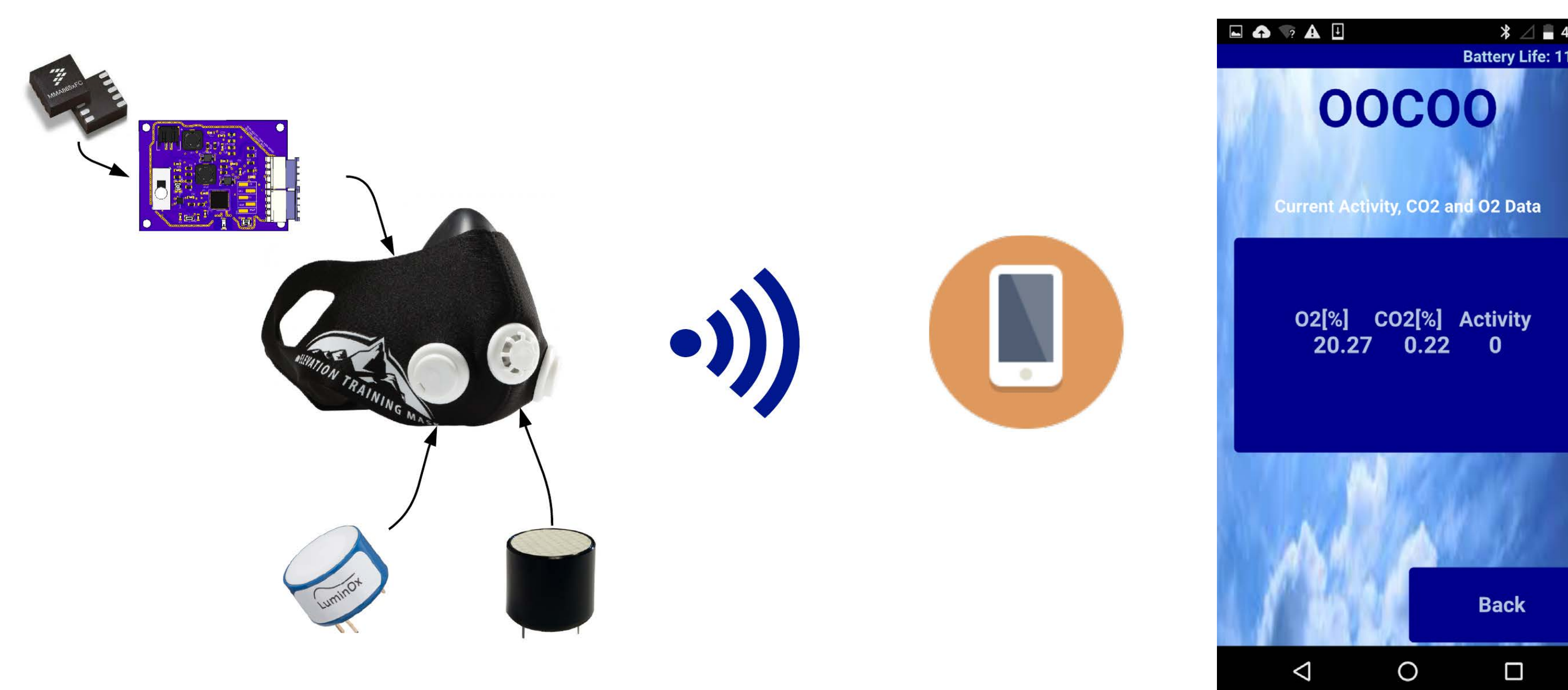
Figure 1. System Overview. The data gathered from the sensors are sent to the smartphone application via Bluetooth.
