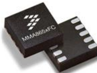
Figure 3: Freescale MMA8652FCR1 Accelerometer
