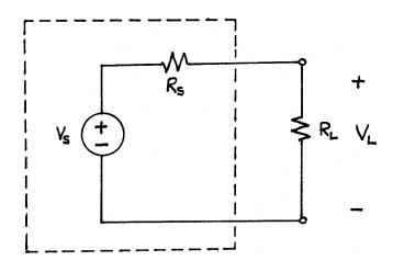
The internal resistance  $R_s$  is 50  $\Omega$ . In the default state of the function generator, it is assumed that the termination, or load resistance  $R_L$  is also 50  $\Omega$ . From the voltage divider relationship, the load voltage  $V_L = V_s/2$ . The displayed voltage  $V_D$  is  $V_s/2$  and thus,  $V_D = V_L$ .
