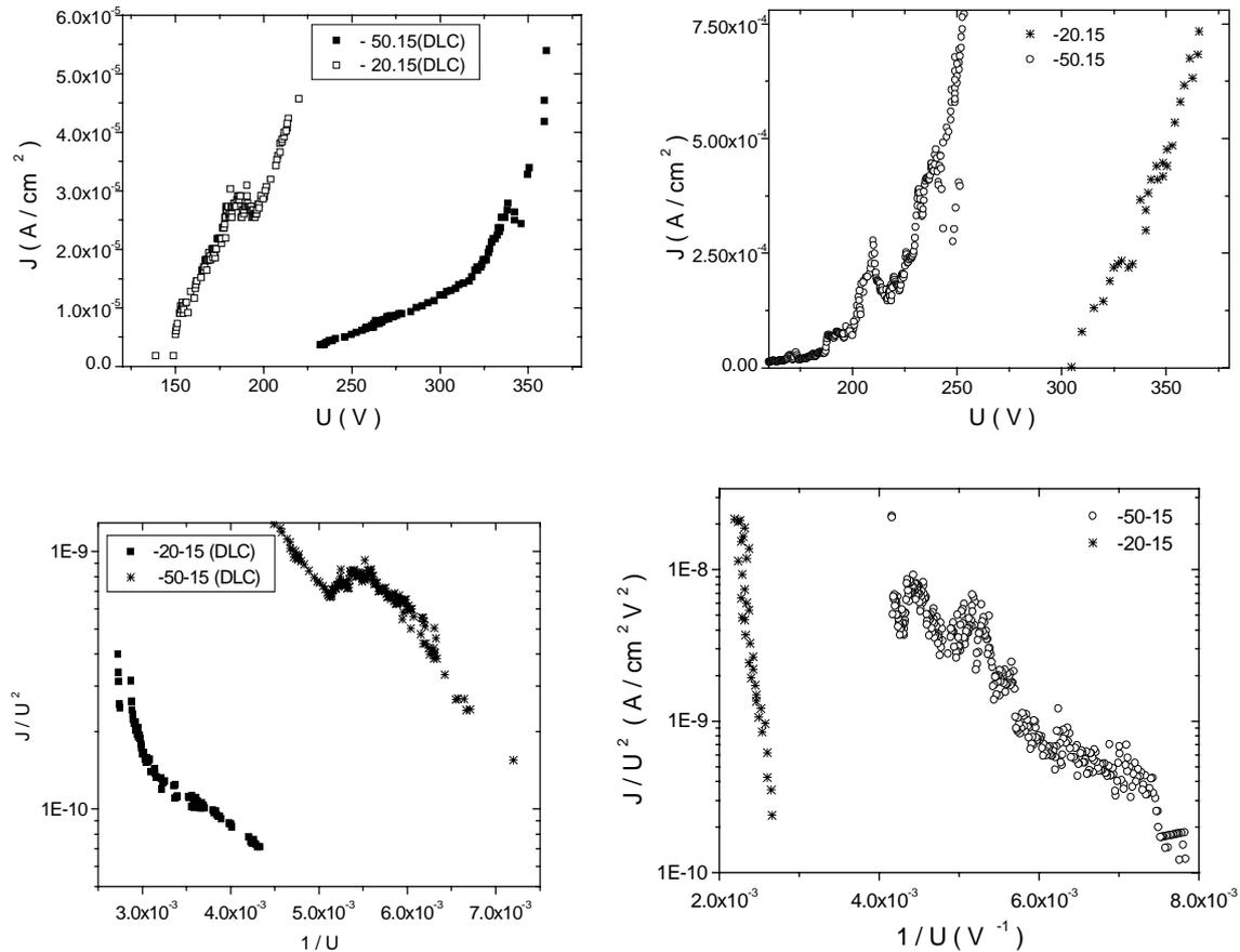
**Figure 2.** Current-voltage (upper graphs) and Fowler-Nordheim (lower graphs) characteristics of electron field emission from Si tips arrays with PS layer covered with DLC (left) and without DLC coating (right). The two regimes of PS formation are: 20 and 50 mA/cm<sup>2</sup>, both for 15 s.
