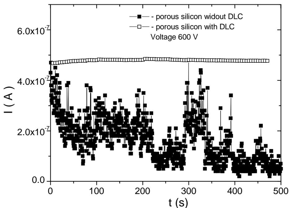
**Figure 4.** Time stability of electron field emission from Si tips with porous silicon layer.
