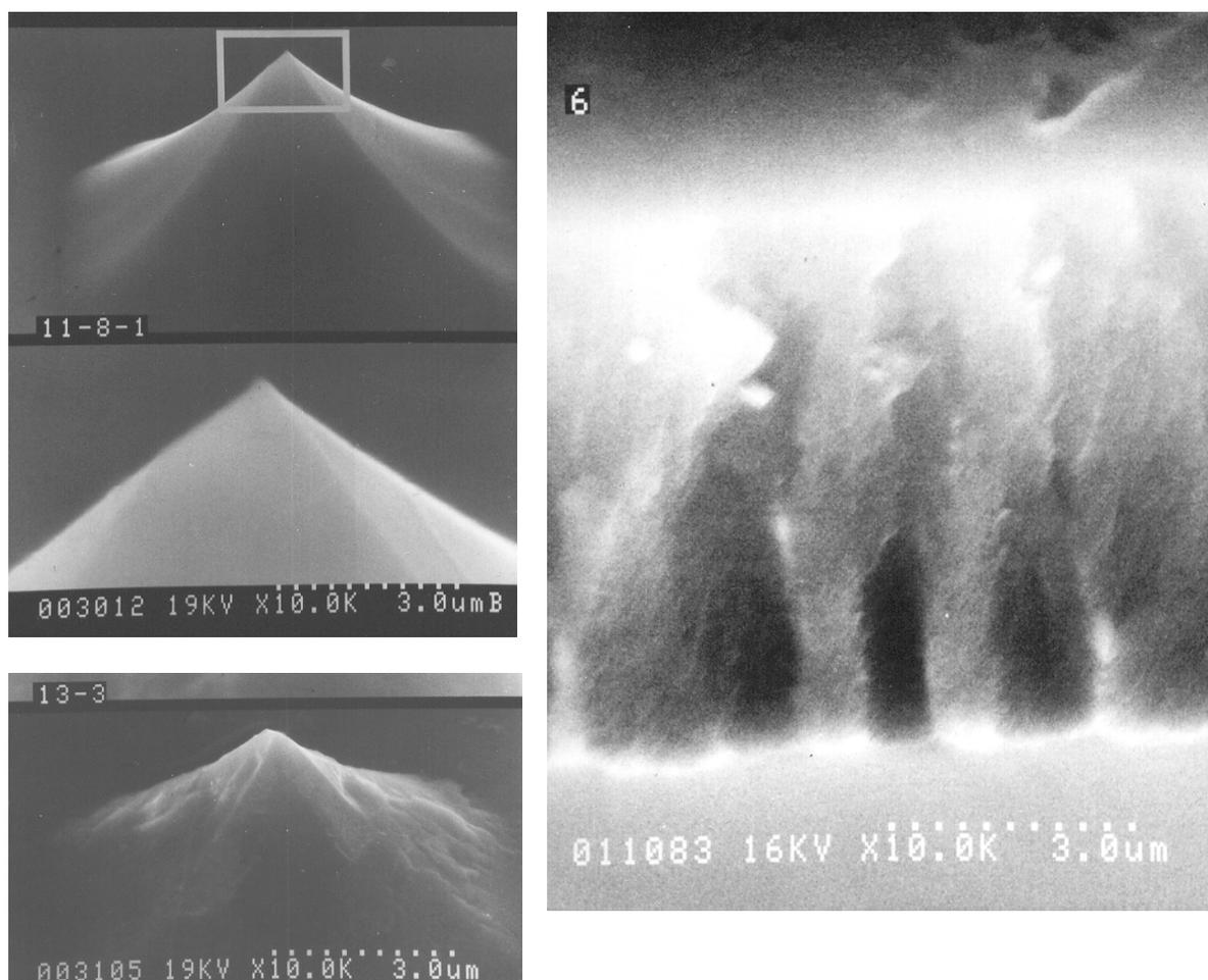
**Figure 1.** SEM micrographs of silicon tips without (a) and with PS layer (b). (c) – enlarged image of the PS layer.
