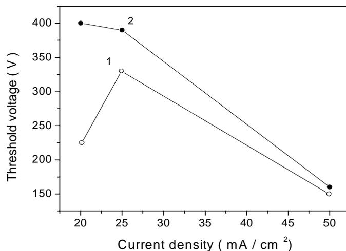
**Figure 3.** Dependence of the threshold voltage ( $V_{th}$ ) for Si tip array on the etching current density: (1) tips coated with porous silicon layer; (2) same tips coated with additional DLC layer.
