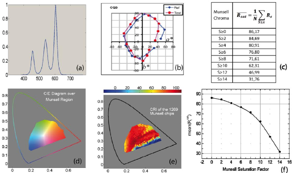
Figure 2.- (a) RGB 3-LED spectrum with good  $R_a$  value. (b) Color differences in an  $a^*b^*$  plot between the LED in (a) and the reference samples used in the Color Quality Scale (CQS). (c) Table showing the results of a CRI-like metric using a complete Munsell set and averaged over the saturation indexes. (d) CIE diagram. (e) Visual representation of CRI over the dense Munsell set. (f) Plot of the data in table (c).
