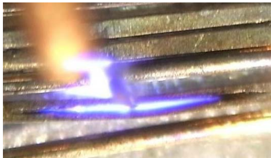
Figure 2. Picture of a MHCD with Argon gas at 800V and 1.2mA
