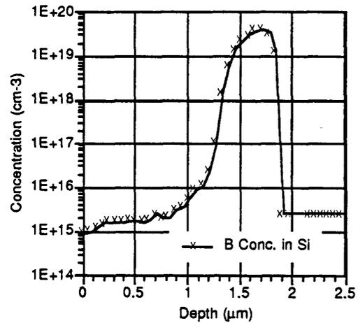
Figure 2: Concentration Profile From SRP Data. Calibrated to B in Si without Ge
