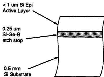
Figure 1: Device wafer films, before bonding and etch-back
