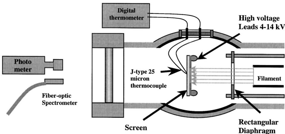
FIG. 1. Test setup for the phosphor efficiency measurements.
