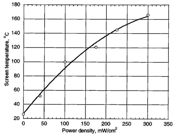
FIG. 2. Experimental relationship between the phosphor screen temperature vs the power density.
