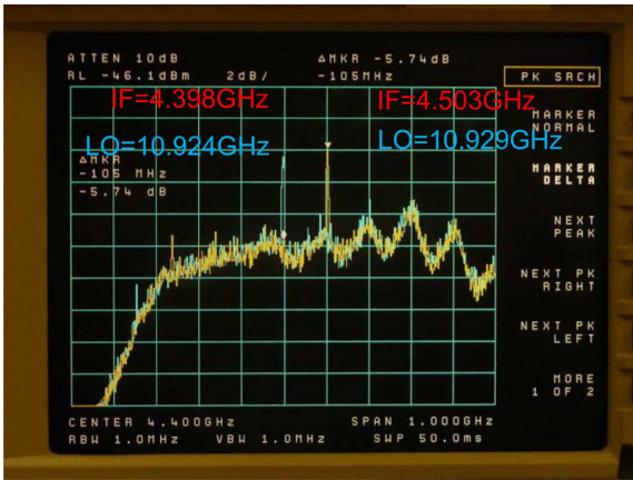
Fig. 14. Fundamental oscillation frequency identified by using high-order (21st) harmonic mixing. 5 MHz shift of LO versus 105 MHz shift of mixer IF suggests the fundamental signal (225.006 GHz) being mixed by the 21st harmonic LO (229.404 GHz or 229.509 GHz) to generate the IF at 4.398 GHz or 4.503 GHz, respectively.
