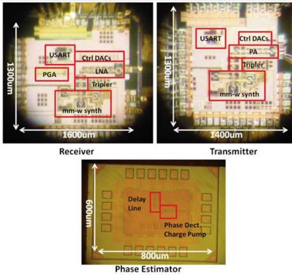
Figure 15.7.7: Die-photos of transmitter, receiver, and DLL chips.
