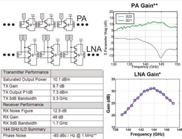
Figure 15.7.2: Schematics and performance of TX and RX mm-Wave front-end. \*LNA gain is simulated values as stand-alone LNA is not available. \*\* PA and ILO are measured from stand-alone test chips.
