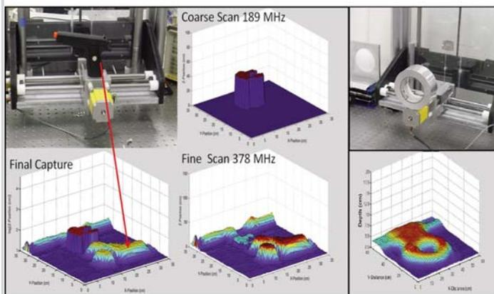
Figure 15.7.5: 3D Image capture showing coarse and fine capture steps of a replica handgun and metallic tape roll at 1m target distance with 2µs integration time. (Z-axis scaling has been adjusted to emphasize the 3D shapes.)
