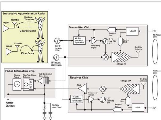
Figure 15.7.1: Principle of operation and block diagram of proposed sub-carrier SAR phase radar.
