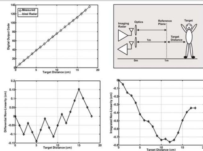
Figure 15.7.4: Target distance response, INL, DNL and spectrum of proposed sub-carrier SAR phase radar. Note the 0.0cm reference plane is set at 1m distance from the radar lenses. The scanning stage is limited to 18cm of travel in Z direction.
