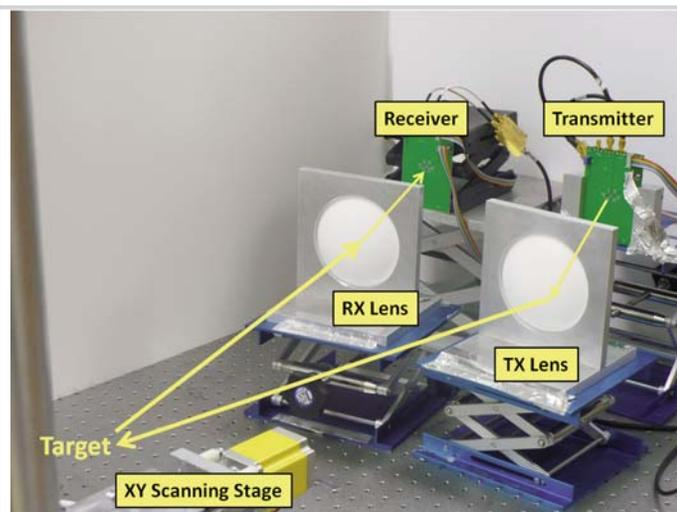
Figure 15.7.3: Test setup photo showing scanning stage and front-end bistatic optics. (note the lenses have been lowered so that TX and RX are visible in the picture.)
