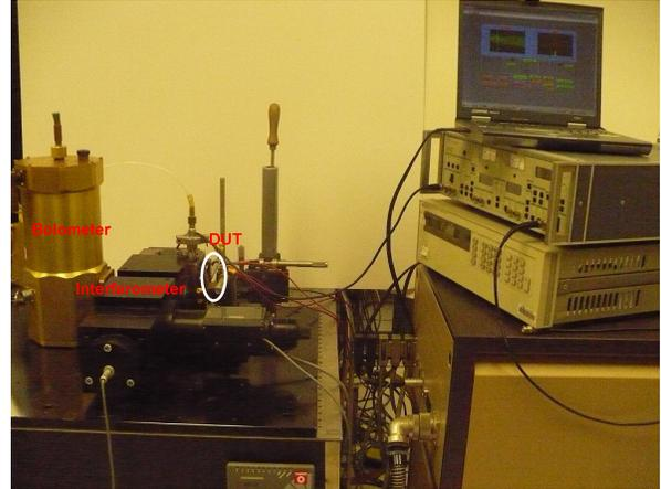
Fig. 4 Quasi-optical setup for measuring terahertz signal outputs.
