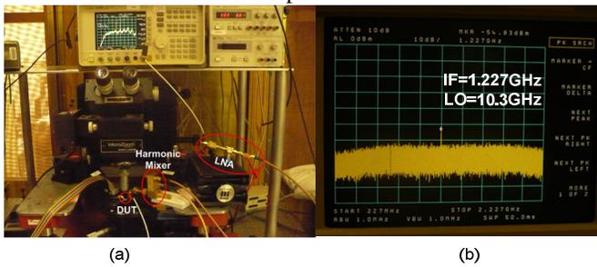
Fig. 3 (a) Setup to measure fundamental resonant frequency ( $f_o$ ) with an external LO and a harmonic mixer; (b) Measured fundamental oscillation at 217.5GHz (or roughly 0.22THz).
