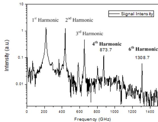
Fig. 5 Measured signal spectrum through Michelson interferometer.
