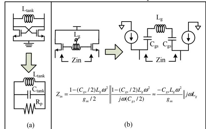
Fig. 2 Stacking resonant tank consisting of: (a) Regular tank at the bottom with  $L_{tank}$  shunt cross coupled drains and its equivalent circuit; (b) Negative-resistance parallel tank shunt between the gates of cascode devices at the top and its equivalent circuit.
