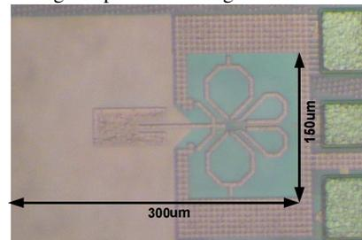
Fig. 6 Die photo of terahertz oscillator with on-chip antenna.
