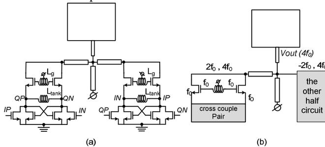
Fig. 1 (a) Terahertz oscillator with stacking resonator tank and on-chip antenna; (b) Illustration of boosted 4<sup>th</sup> order harmonic at expense of suppressed odd-order and 2<sup>nd</sup> order harmonics.
