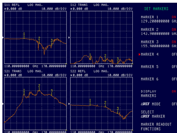
Figure 9. Measured S parameters under 2V supply
