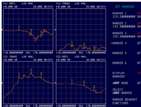
Figure 8. Measured S parameters under 1.4V supply
