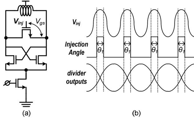
Fig. 1. (a) Voltage injection prescaler circuit insertion and (b) its effective injection angle  $\theta_1$  indicated around prescaler output's crossing period.
