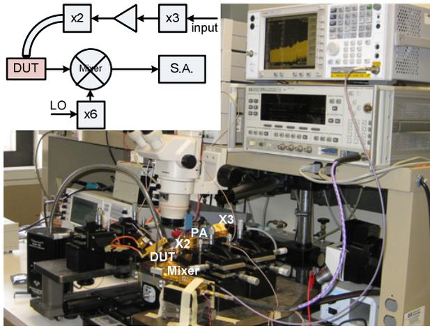
Fig. 4. Measurement setup.
