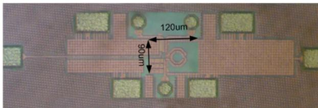
Fig. 8. Die photo of CMOS prescaler with time-interleaved dual injection locking.
