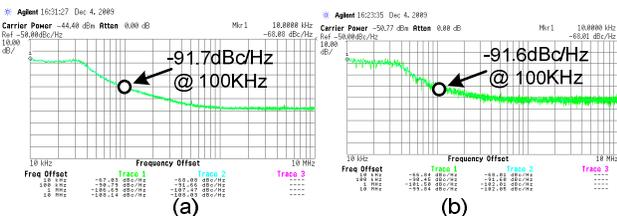
Fig. 7. Measured output phase noises of (a) first divide, (b) second divider.
