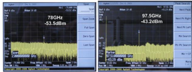
Fig. 5. FD-V1 measured results (a) input sensitivity (b) output spectrums at lowest/highest input frequencies of 156/195GHz.
