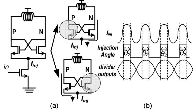
Fig. 2. (a) Current injection prescaler circuit insertion and (b) its effective injection angle  $\theta_2$  indicated around prescaler output's positive (or negative) peaking period.
