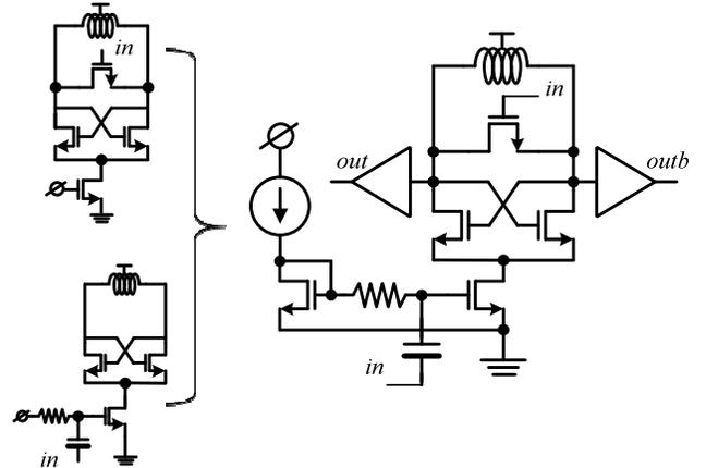
Fig. 3. A time-interleaved injection locking prescaler with enhanced injection angle.
