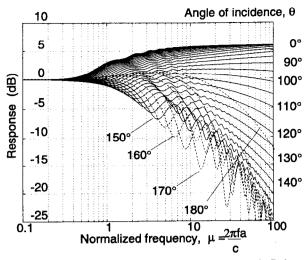
Figure 1: Magnitude response for a source at infinity
