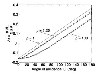
Figure 7: Normalized arrival time for three different ranges
