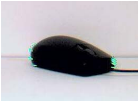
Figure 4. 42 and 152 Features are selected on a simple object with FS-FIX and FS-AUTO, respectively.
