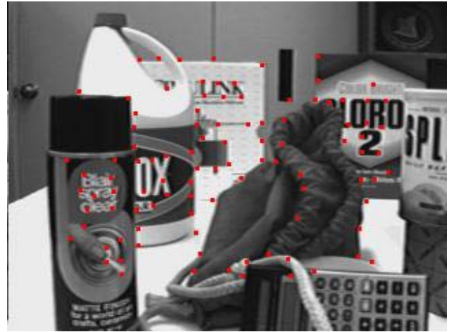
Figure 1. Feature selection algorithm performed on a sample image. Selected features are denoted by small dark squares.
