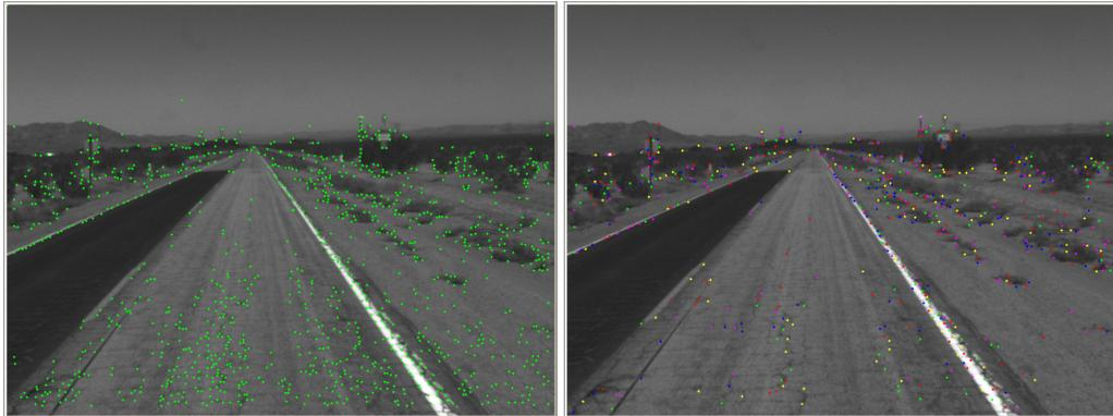
**Fig. 4.** Left: FPGA selection output, sample frame. There are 1162 feature selected, obtained with threshold parameter  $\lambda_t = 50$ . Right: Tracking output, sample frame, obtained with selections in figure 4 as input. Tracks are displayed as dots of different colors, their total number in this frame is 562.
