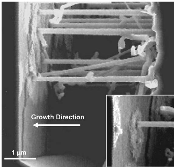
Fig. 1. Representative cross-sectional scanning electron micrograph of gold-catalyzed silicon nanowires bridged between two vertical sidewalls of a 5 μm wide trench. The inset shows the impinging end of a bridging nanowire and the disc-like deposit formed on the “opposing” sidewall. The nanowires were grown at 680 °C for 30 min at 10 Torr using 15 sccm SiH<sub>4</sub>, 15 sccm HCl, and 3 slm H<sub>2</sub>.
