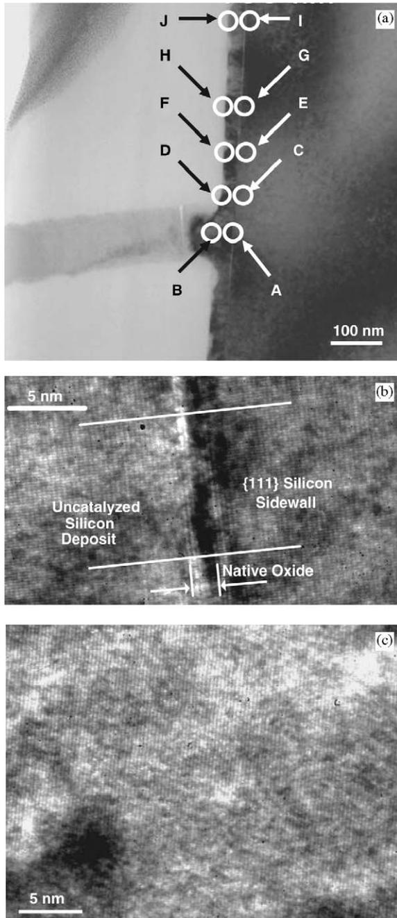
Fig. 3. (a) Low-magnification, bright-field TEM image of the impinging-end region of a bridged silicon nanowire (the different regions on the impinging-end sidewall have been labeled A through J). (b) HRTEM image of region A, the interface region of the uncatalyzed silicon deposit and the impinging-end sidewall. (c) HRTEM image of the neck region (labeled as region B in (a)) that forms at the impingement location of the nanowire with the opposing sidewall.
