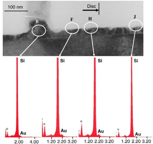
Fig. 4. EDX spectra collected from different regions on the opposing sidewall (letters correspond to positions indicated in Fig. 3.)
